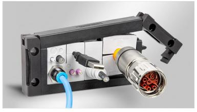
The KEL-FA range is a compact system to route and seal pre-terminated cables as well as conduits or pneumatic hoses utilising KT series grommets. After populating the entry frame with grommets and cables, the cover is put on and the two clamping levers are locked with the lower part by pressing them down. The twist-proof construction of the KEL-FA enables intuitive assembly. Routing and sealing with IP54 / UL Type 12 for cable diameters from 1 to 35 mm.
